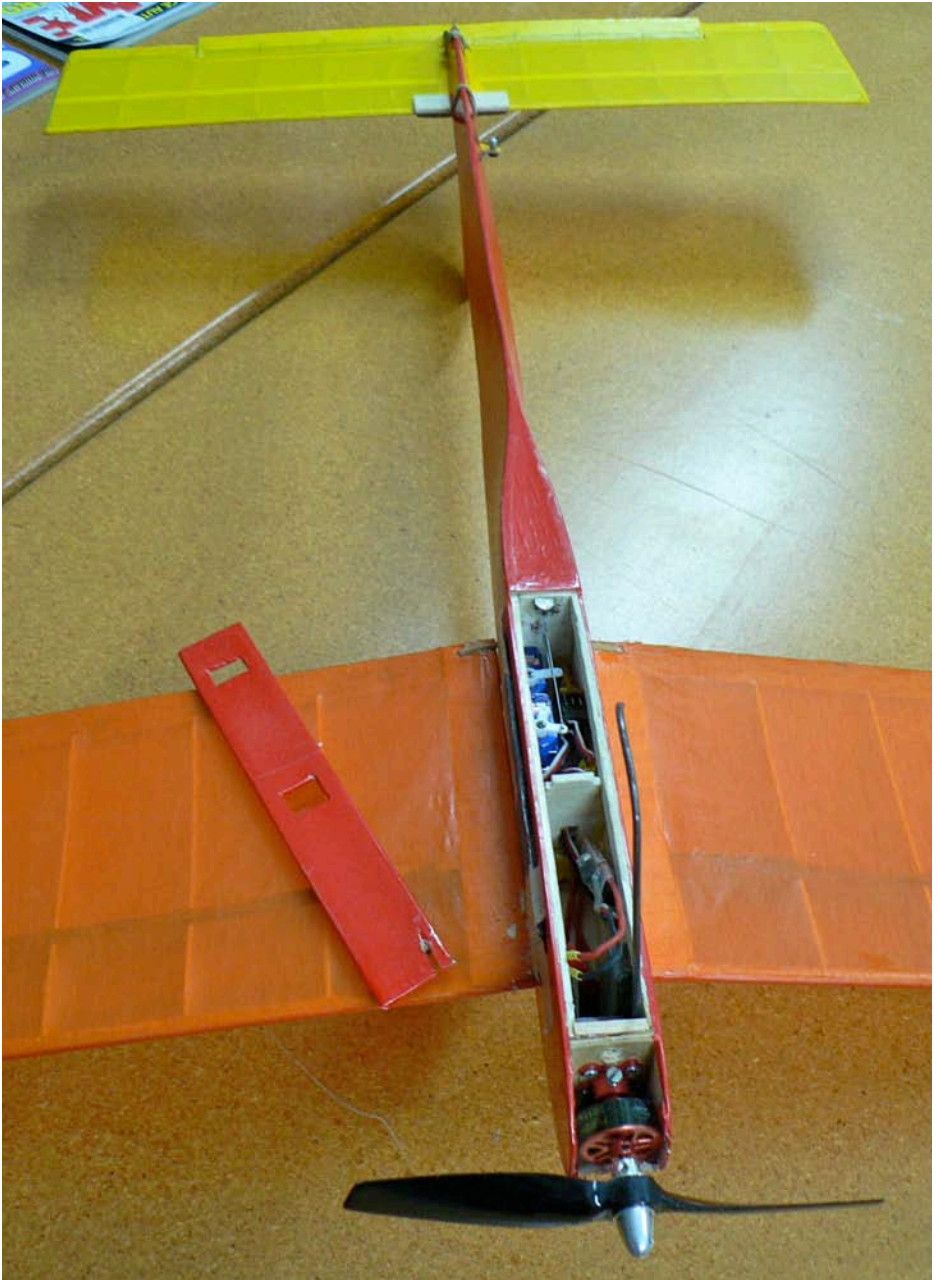
Above: Angus Macdonald turned over his Jumpin Bean, to reveal the tight space for battery and RC gear.
